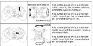
Tip: please send aircraft to fly to 1.5 meters or more height, then the rolling manipulation.
