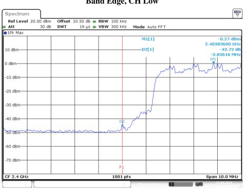
EDR Hopping Mode (8DPSK) Band Edge, CH Low
