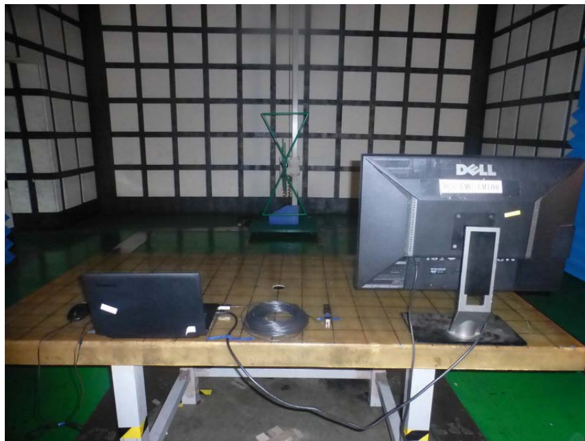
Photograph 4: Radiated Emission Test Configuration, (Below 1GHz) Back
