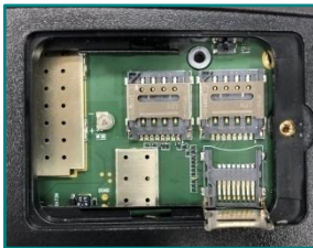
Figure 2-4 unlock the card slot cover and insert the microSD card into the slot.
