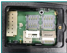
Figure 2-7 unlock the card slot cover(s) and insert the SIM card into the slot.
