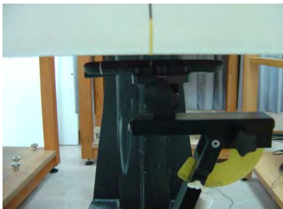
Fig.7 EUT front to flat phantom
