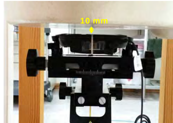
Fig.13 EUT front with headset to flat phantom
