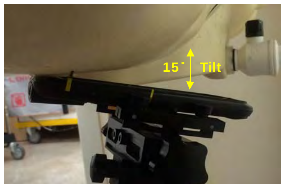
Fig.3 Right Head Section / Cheek-Touch Position
