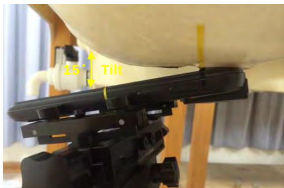
Fig.6 Left Head Section / Ear-Tilt Position(15°)
