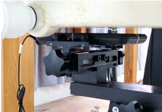
Fig.13 EUT front with headset to flat phantom
