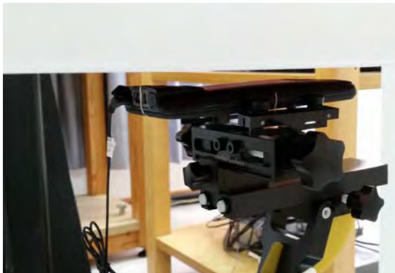
Fig.14 EUT back with headset to flat phantom
