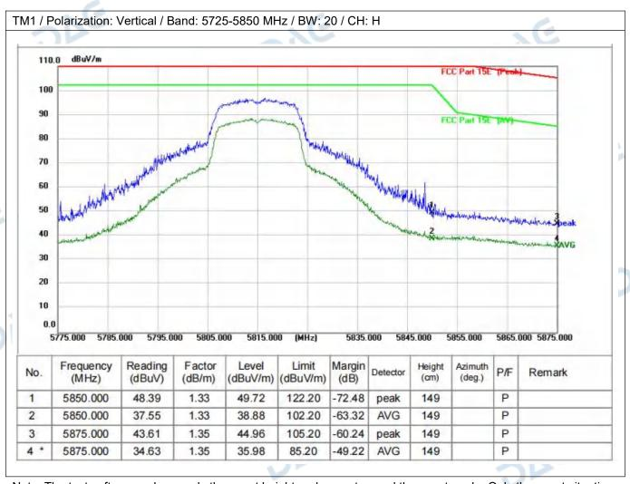
Note: The test software only records the worst height and cannot record the worst angle. Only the worst situation is displayed in the test report.
