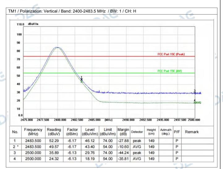
Remark: The test software will only record the worst test angle and height, and only the worst case will be displayed in the test report.
