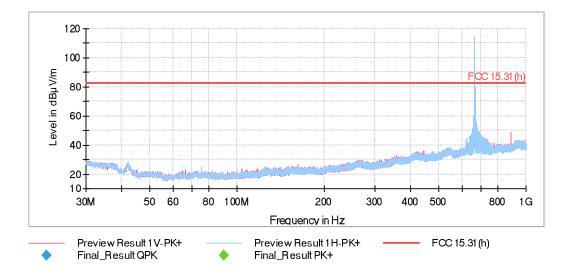
The peak on the left above the limit is the carrier frequency LTE Cat-M1 Band 71 (668 MHz).
