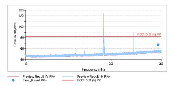
The peak above the limit is the carrier frequency LTE Cat-M1 Band 25 (1882.5 MHz).
