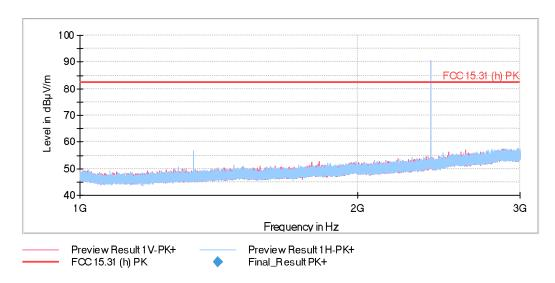
The peak on the right above the limit is the carrier frequency Bluetooth Low Energy (2402 MHz).
