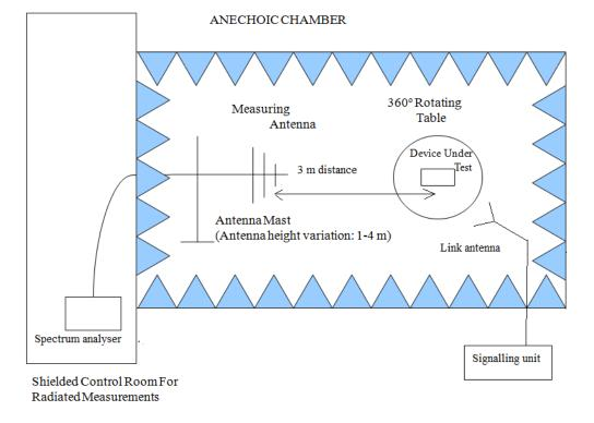
Radiated measurements between 1 GHz and 17 GHz.
