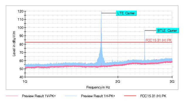
The peak above the limit is the carrier frequency LTE Cat-M1 Band 66 (1770 MHz). The peak above the limit is the carrier frequency Bluetooth Low Energy (2440 MHz).
