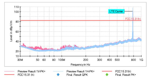
The peak above the limit is the carrier frequency LTE Cat-M1 Band 13 (779.5 MHz)
