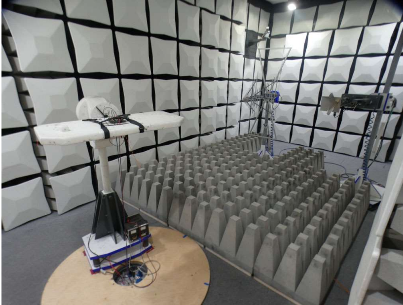
Photo 1: Test setup for radiated measurements above 1GHz
