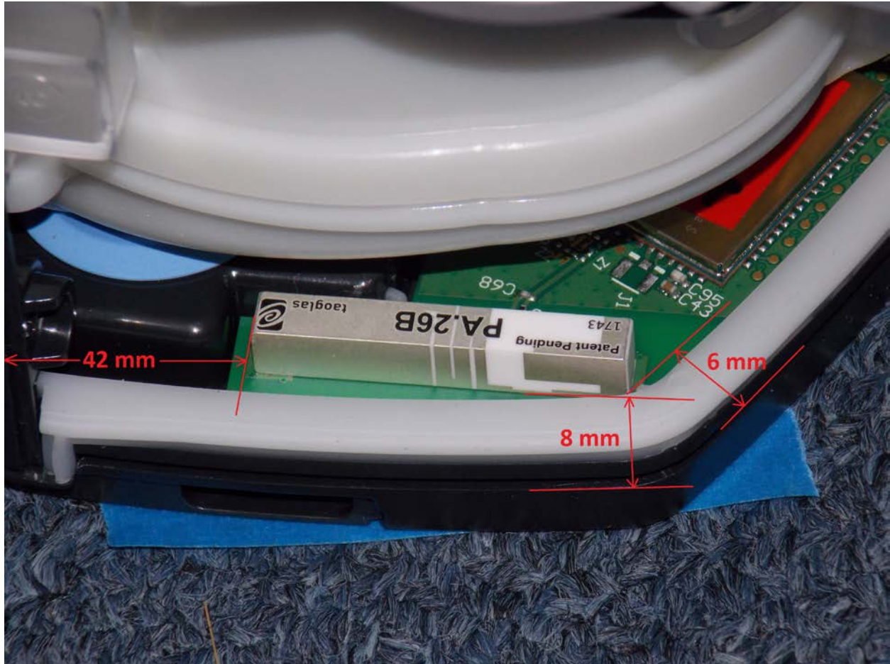
Antenna Distances in Device to Back Top and Bottom Antenna Size 35mm x 5mm x 6mm
