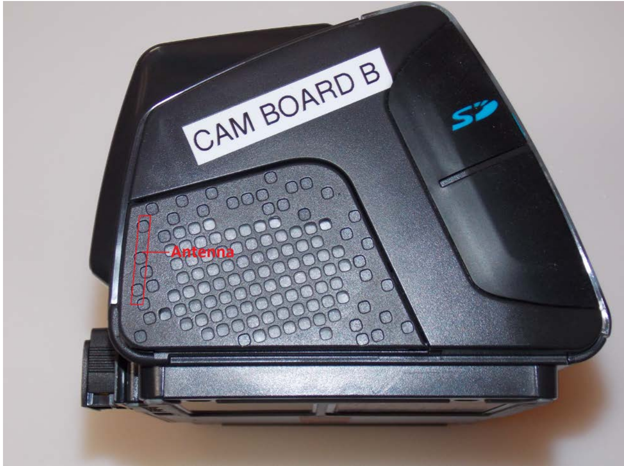
Antenna Location on End
