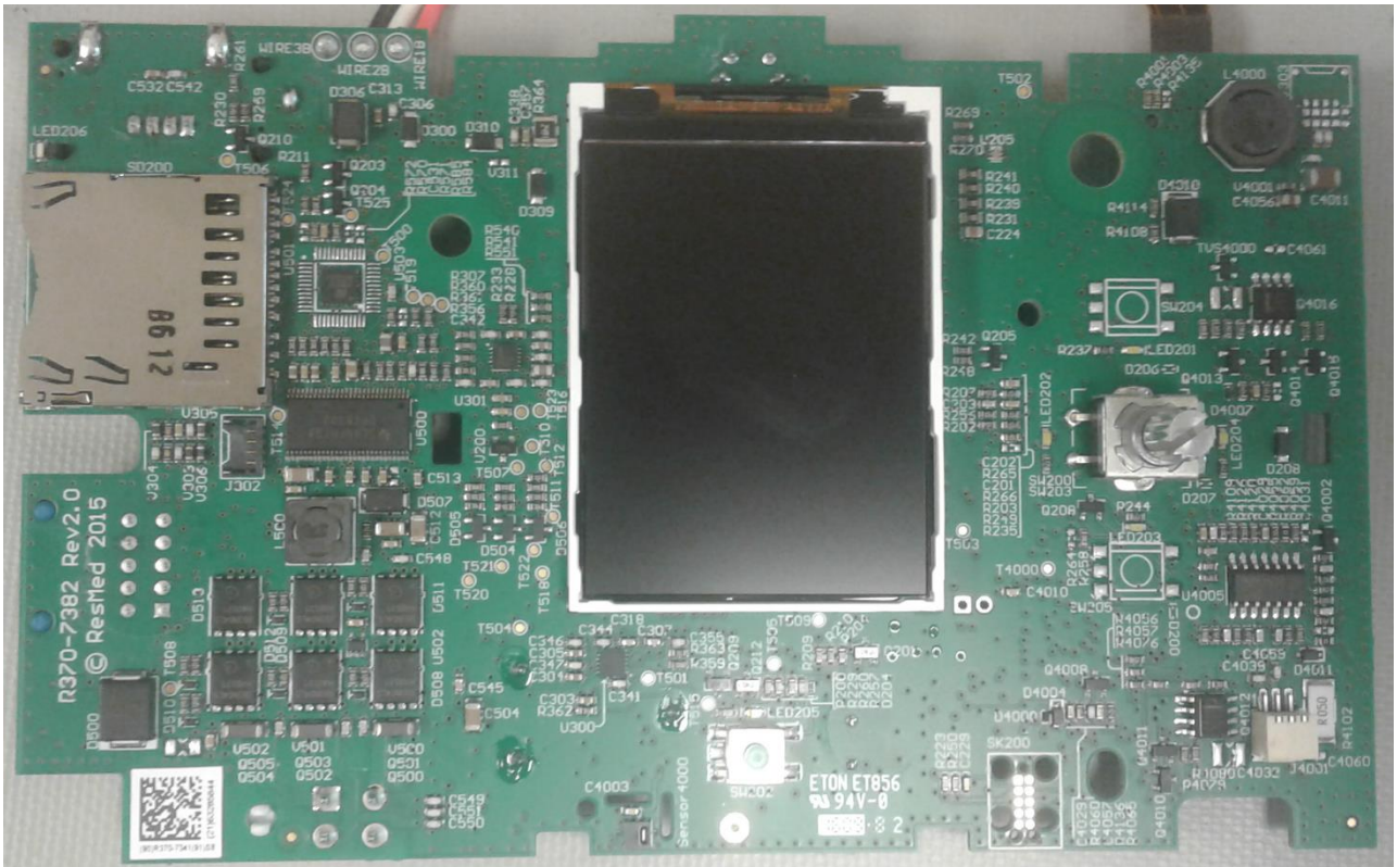
Display Side of Flow Generator Mother Board
