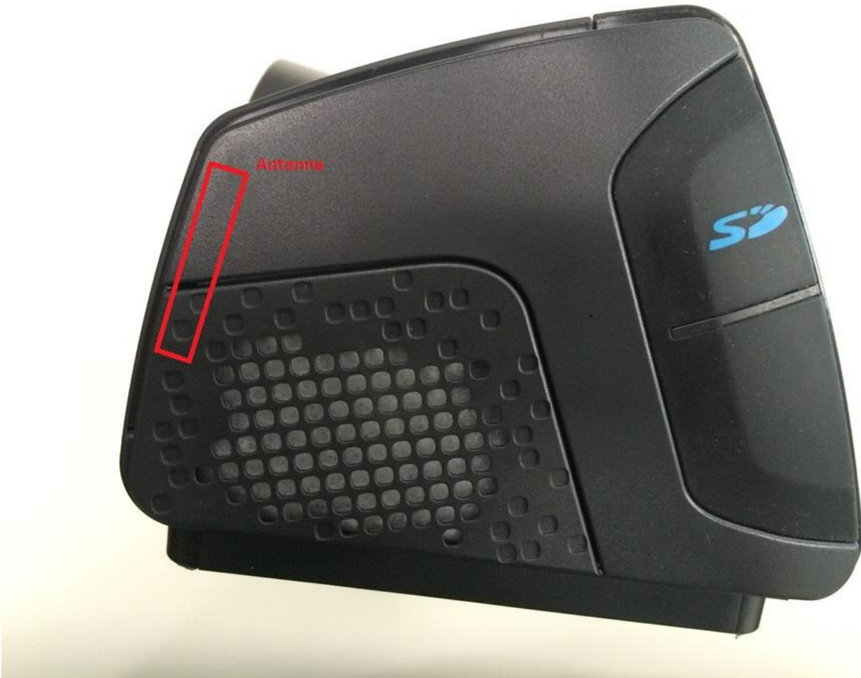
Cellular Antenna location
