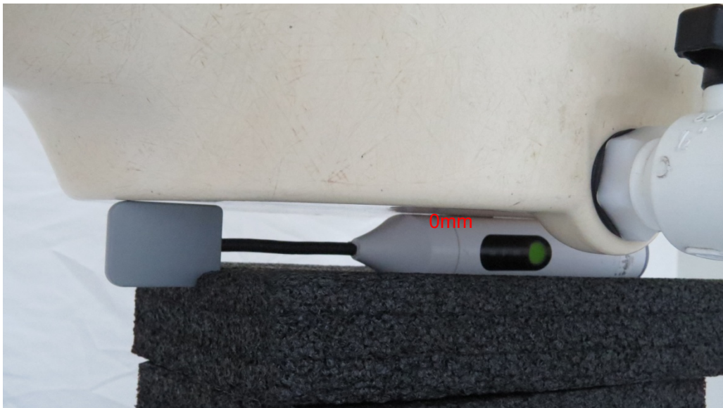
Picture 4: Right Edge, the distance from handset to the bottom of the Phantom is 0mm
