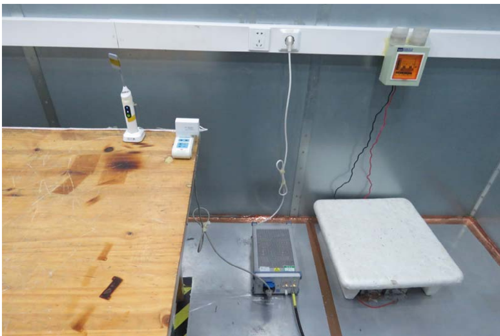
Picture 2 Conducted Emission Test Setup
