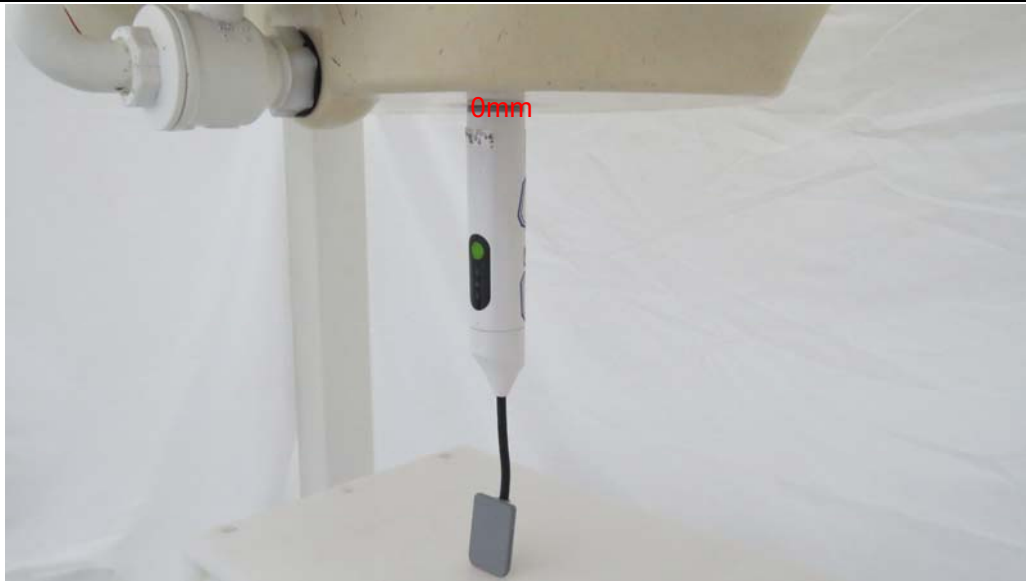
Picture 5: Bottom Edge, the distance from handset to the bottom of the Phantom is 0mm
