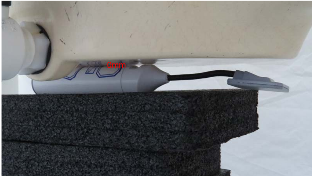
Picture 1: Back Side, the distance from handset to the bottom of the Phantom is 0mm
