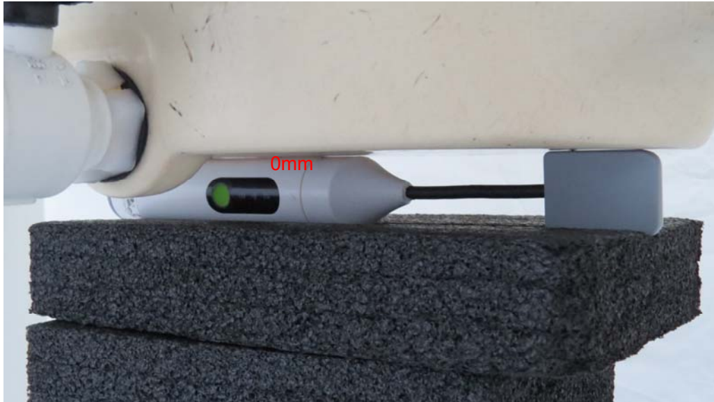
Picture 3: Left Edge, the distance from handset to the bottom of the Phantom is 0mm
