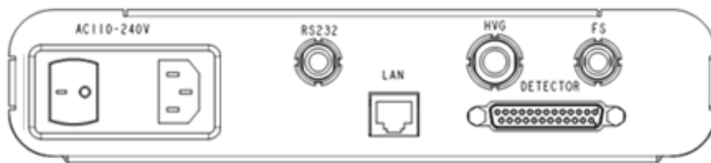
Rear View of Control Box
