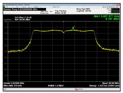
PSD 802.11ac(VHT20) 5745MHz
