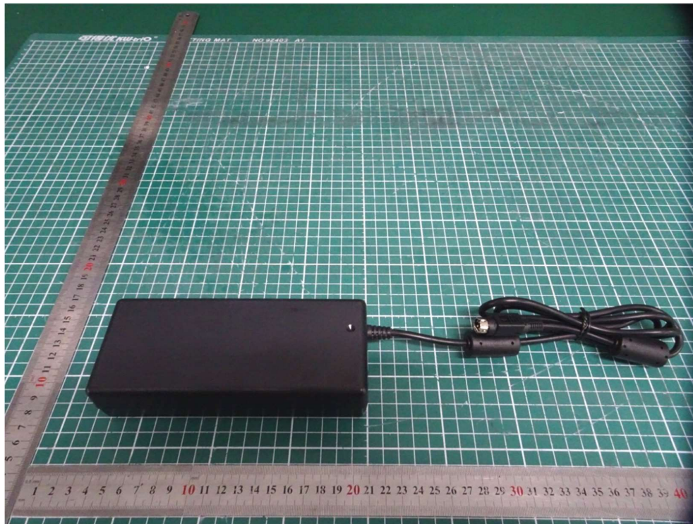
c: Switching Power Supply
