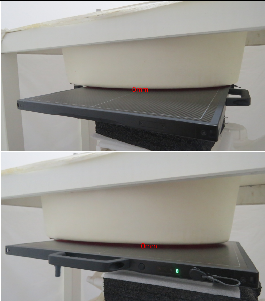
Picture 1: Front Side, the distance from handset to the bottom of the Phantom is 0mm
