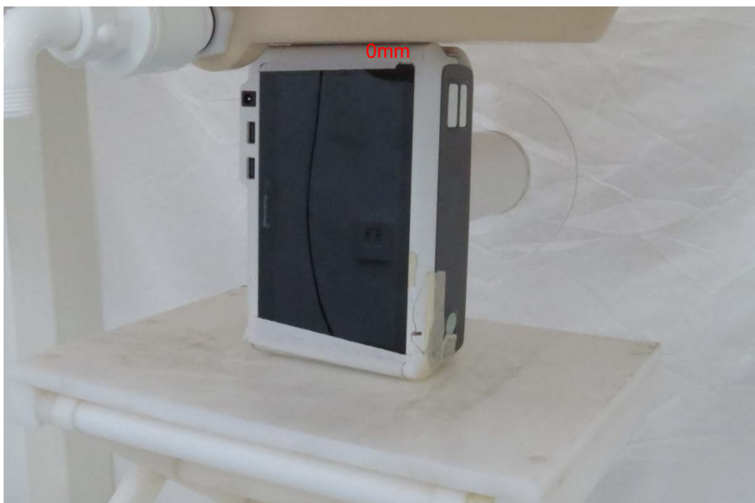
Picture 2: Left Edge, the distance from handset to the bottom of the Phantom is 0mm.
