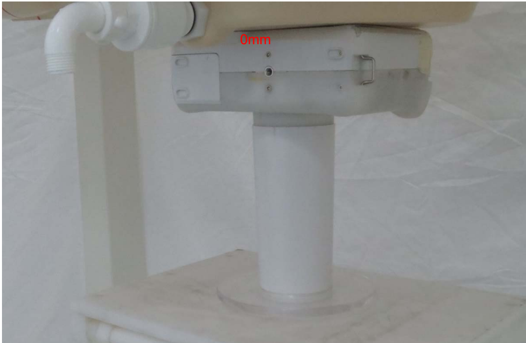
Picture 1: Front Side, the distance from handset to the bottom of the Phantom is 0mm.
