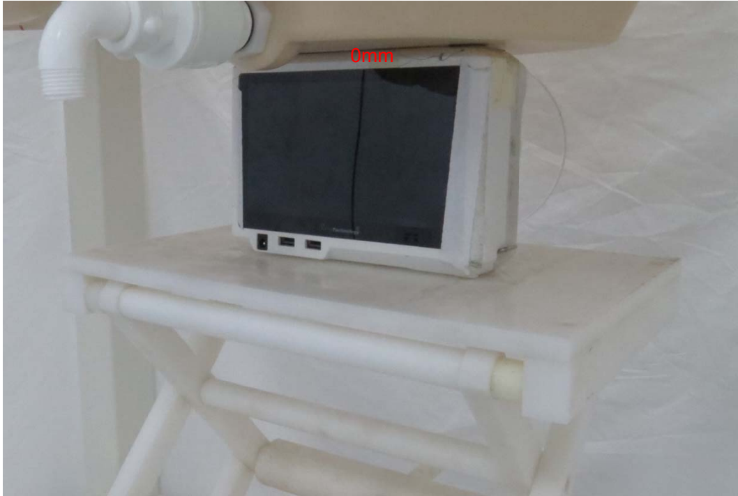
Picture 3: Top Edge, the distance from handset to the bottom of the Phantom is 0mm.
