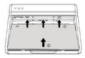
3. Press the battery down into the battery compartment.
