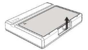
2. Insert battery into battery charger in the orientation shown below.
