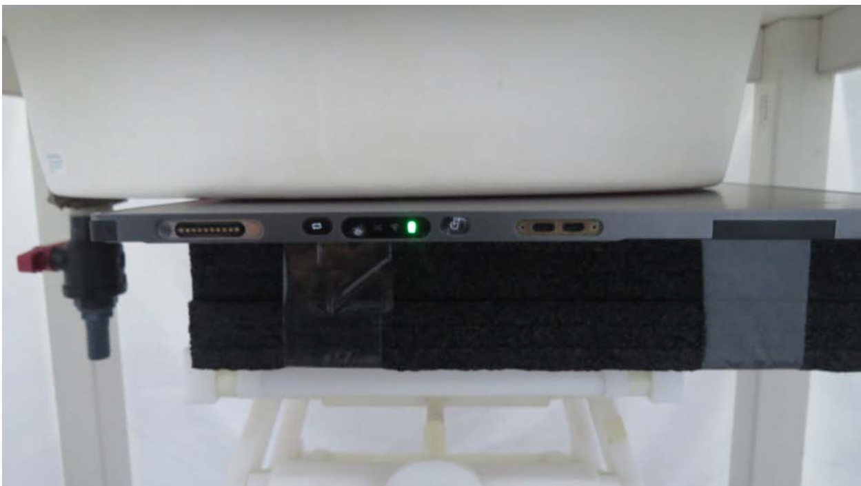
Picture 2: Front Side, the distance from handset to the bottom of the Phantom is 0mm (Scan 2)
