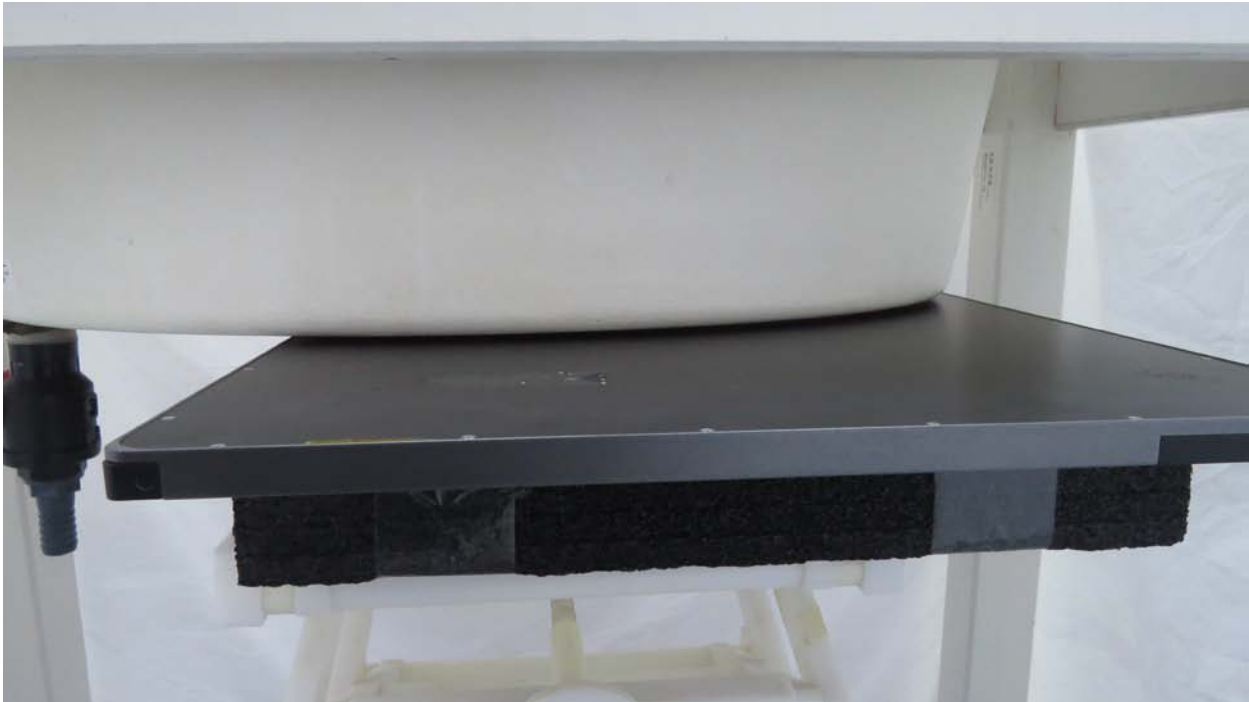
Picture 1: Front Side, the distance from handset to the bottom of the Phantom is 0mm (Scan 1)
