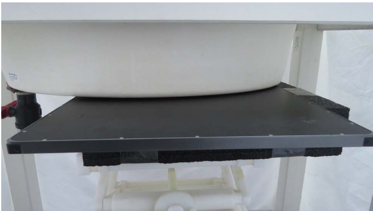
Picture 4: Front Side, the distance from handset to the bottom of the Phantom is 0mm (Scan 4)
