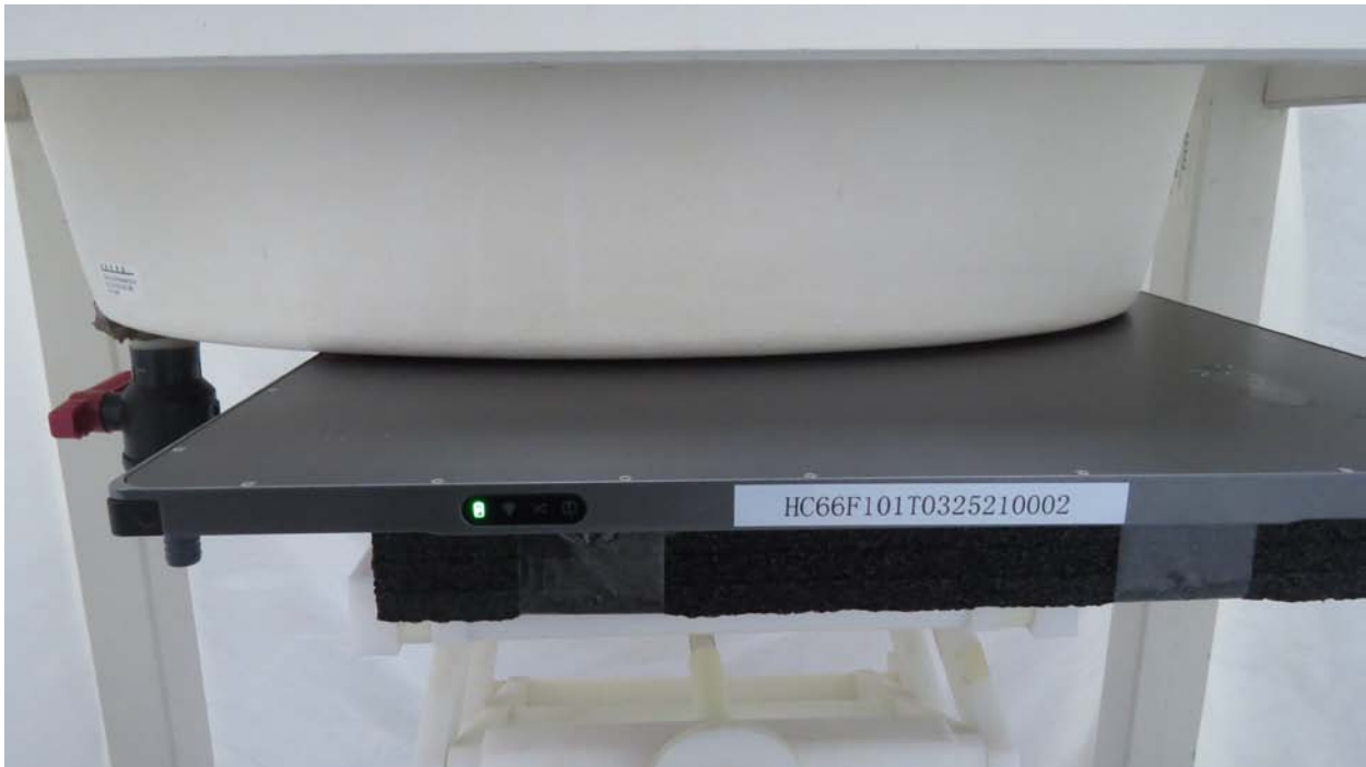
Picture 3: Front Side, the distance from handset to the bottom of the Phantom is 0mm (Scan 3)
