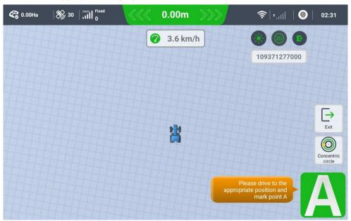
Input the minimum radius between adjacent circles, or drive the car to the target position and get the distance
