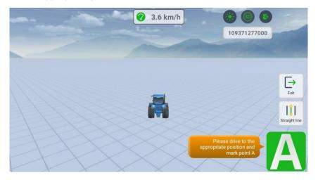
After that, drive to *Point B*, and the distance from A to B should greater than 10 meters
