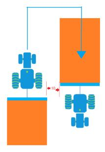
For example, in the farm tool settings picture, the actual width of the farm tool A is 6M, the handover row B is set to 0M, and the offset value C is 0. However, when working in the second row, the tractor veers to the right. If the value is 10CM, then in the "Quick Handover Adjust" on the right side of the main interface of the software, please select "Right" and enter "10CM" as the value to complete the quick adjust.
