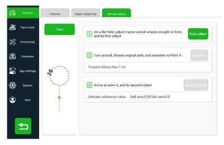
Attitude adjust is to obtain the calibration value of roll angle and pitch angle of the vehicle. The first step is to click First collect to collect a point as point A.
