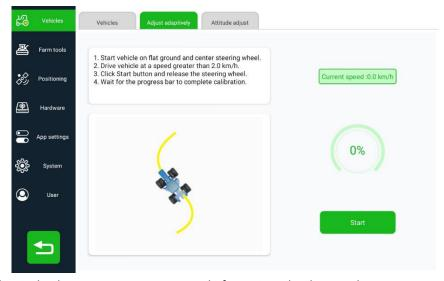
Adjust adaptively obtain proper motor control of steering wheel strength.
