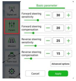
**Forward steering sensitivity:** Obtained from Adjust parameter adaptively. Control how fast the steering wheel turns. The higher the value, the faster the steering wheel turns. Default value is 30
