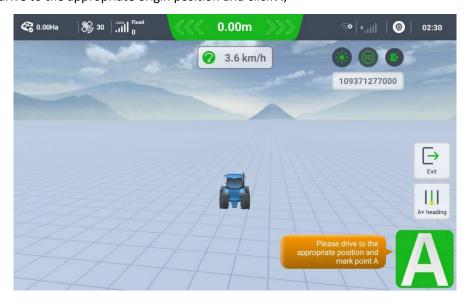
The vehicle will automatically determine the angle between the current heading and the north direction. You can also enter the angle value independently.
