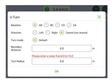
When the tractor is in the area, turn on the autosteer, and when it is about to reach the intersection of the Job line and the boundary, it will automatically turn around according to the set parameters.
