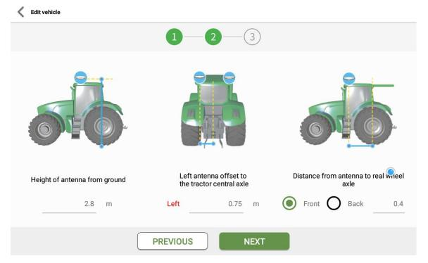
"Height of antenna from ground": Vertical distance from antenna to ground.
