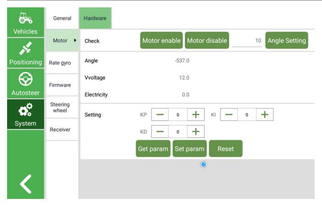
(1) Click *Motor*, you can check whether the communication of the motor is normal through *Motor enable*, *Motor disable* and *Angle Setting*.
