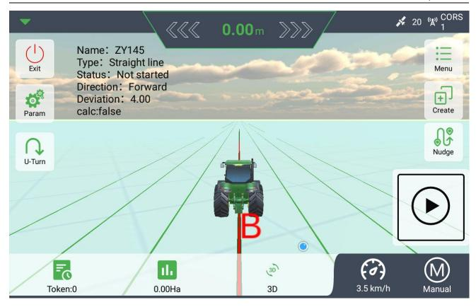
Each time you stop automatic driving, the *U-turn* around option will appear in the lower left corner. You can select the turning direction for the next driving as required.
