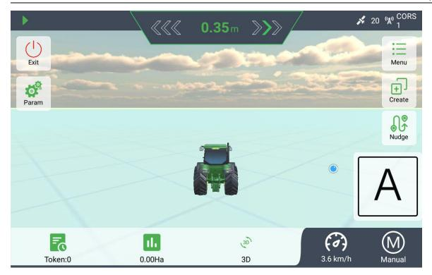
Hold the steering wheel to drive tractor to the other end of the field, choose the location and stop, click **B** button, and the AB line will be confirmed. The lateral deviation value will also return to 0 (The distance between point A and point B is at least 20 m)
