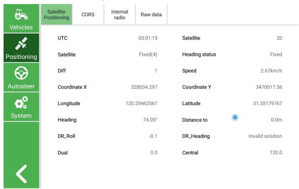
(1) Click *Internal radio* to configure radio information and get a fixed solution. Choose the correct channel to receive the correction data from base station.
