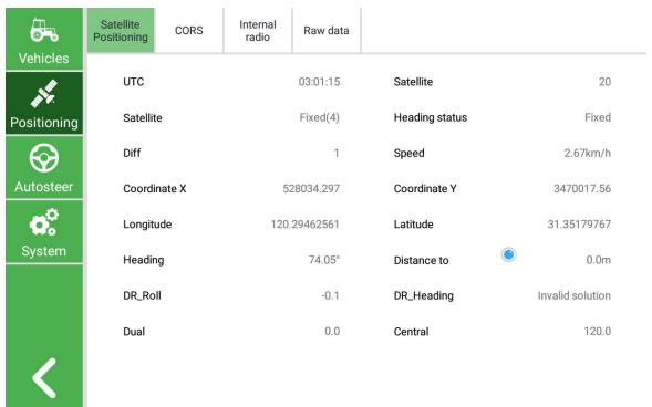
(2) Click *Internal radio* to configure radio information and get a **fixed** solution. Choose the correct channel and protocol. Then click **setting** >**read** to receive the correction data from base station.
