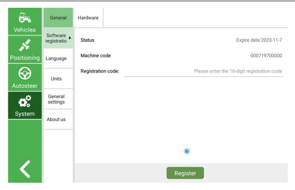
If you want to register, you need to connect the GNSS antenna first. When the receiver has successfully received the GNSS data, the unregistered device will have a pop-up window prompting to register.
