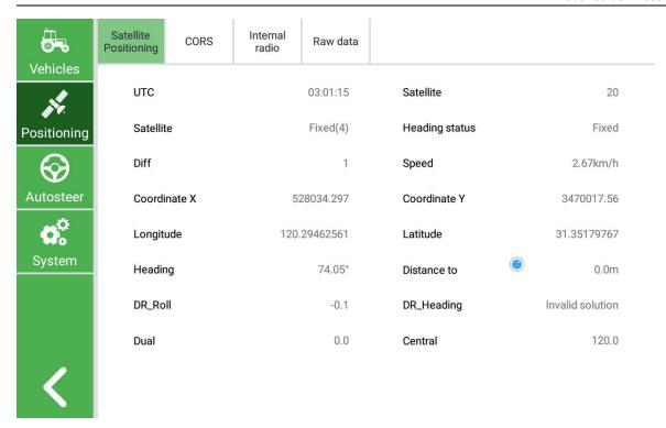
(1) Click **Satellite Positioning** to check satellite positioning status.
