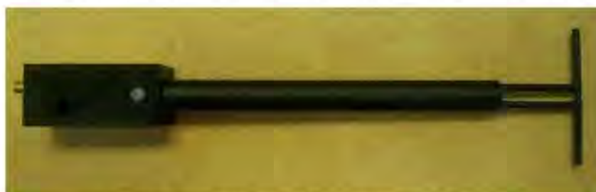
Figure 1 – MVG COMOSAR Validation Dipole
