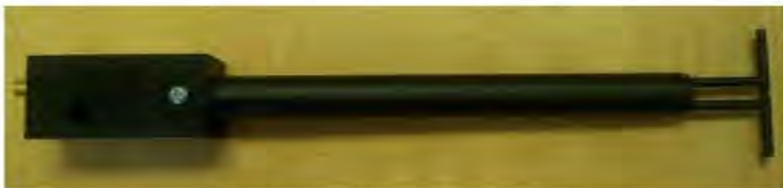
Figure 1 – MVG COMOSAR Validation Dipole
