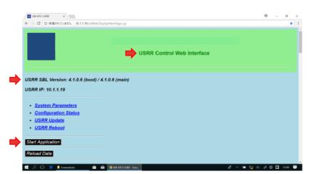
The USRR Control Web Interface is started. (Confirm that it is "USRR SBL Version: 4.1.0.6(boot)/4.1.0.6(main)") Press the "Start Application"
