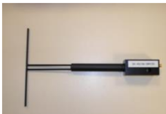
Figure 1 – Satimo COMOSAR Validation Dipole
