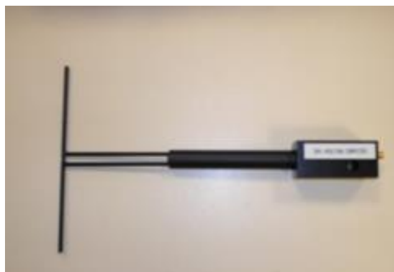
Figure 1 – Satimo COMOSAR Validation Dipole
