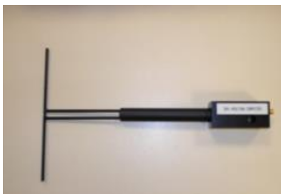
Figure 1 – Satimo COMOSAR Validation Dipole
