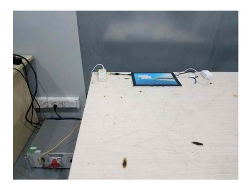
Radiation Emission Test Setup (Below 30MHz)
