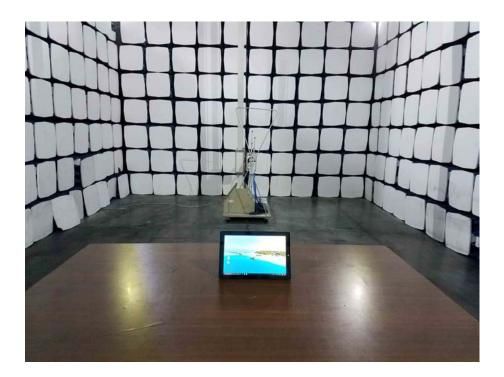
Radiation Emission Test Setup (Above 1GHz)
