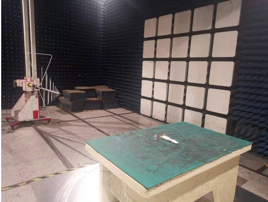
Spurious Emission Test Setup (Above 1GHz)
