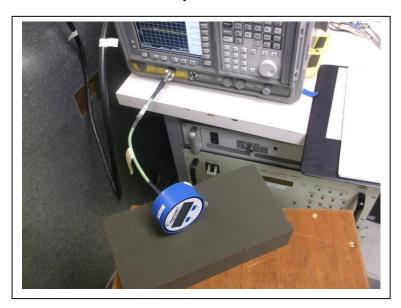
RF Output Power, Conducted Spurious Emissions, Peak Power Spectral Density
