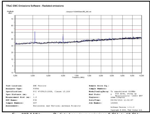
Fc = 927.6 MHz Radiated spurious emissions 5 GHz to 10 GHz
