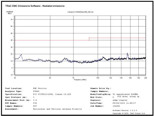
Fc = 927.6 MHz Radiated spurious emissions 30 MHz to 200 MHz
