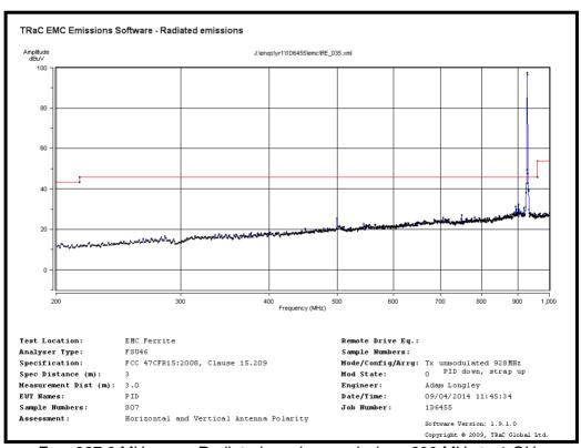
Fc = 927.6 MHz Radiated spurious emissions 200 MHz to 1 GHz
