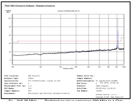
Fc = 915.25 MHz Radiated spurious emissions 200 MHz to 1 GHz
