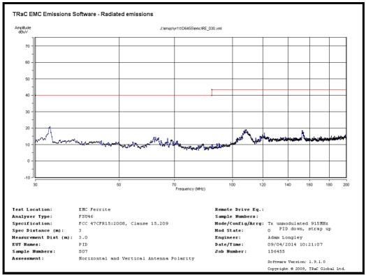
Fc = 915.25 MHz Radiated spurious emissions 30 MHz to 200 MHz
