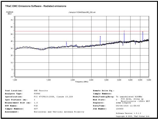
Fc = 927.6 MHz Radiated spurious emissions 1 GHz to 5 GHz
