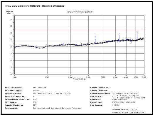
Fc = 915.25 MHz Radiated spurious emissions 1 GHz to 5 GHz
