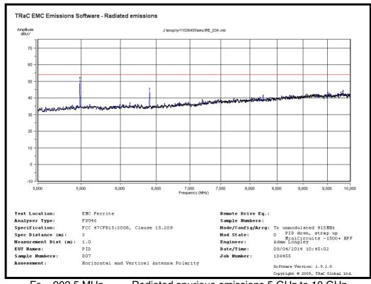
Fc = 902.5 MHz Radiated spurious emissions 5 GHz to 10 GHz
