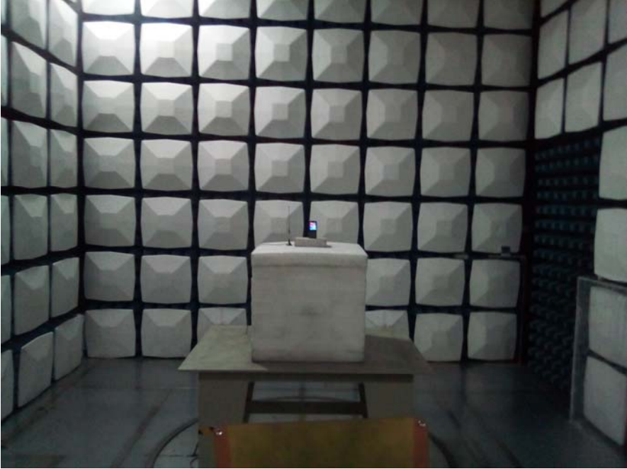
Radiated Emission Above 1GHz View
