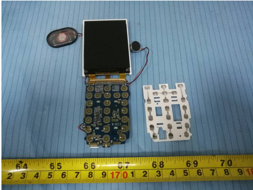
EUT – Main Board Top Shielding off View
