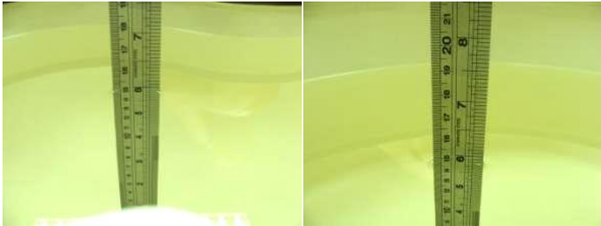
Photo of Liquid Height for Head SAR
