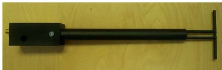
Figure 1 – MVG COMOSAR Validation Dipole
