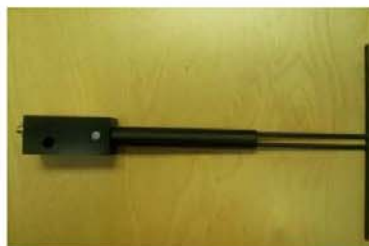
Figure 1 – MVG COMOSAR Validation Dipole
