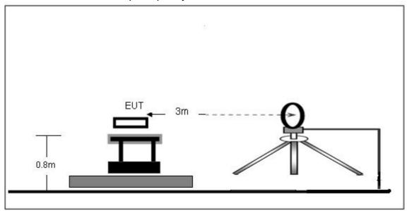
(B) Radiated Emission Test-Up Frequency 30MHz~1GHz
