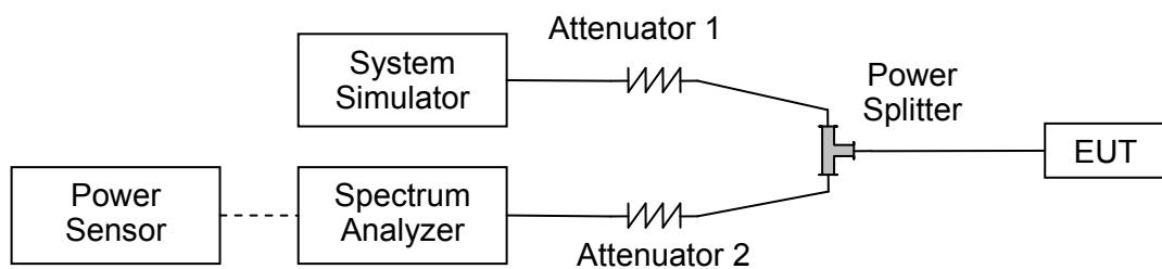
The EUT is coupled to the Spectrum Analyzer (SA) and the System Simulator (SS) with Attenuators through the Power Splitter; the RF load attached to the EUT antenna terminal is 50Ohm; the path loss as the factor is calibrated to correct the reading. The EUT is commanded by the SS to operate at the maximum output power. A call is established between the EUT and the SS.
