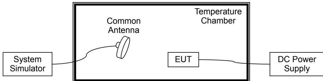
The EUT which is powered by the DC Power Supply directly, is located in the Temperature Chamber. The EUT is commanded by the System Simulator (SS) to operate at the maximum output power. A call is established between the EUT and the SS via a Common Antenna.
