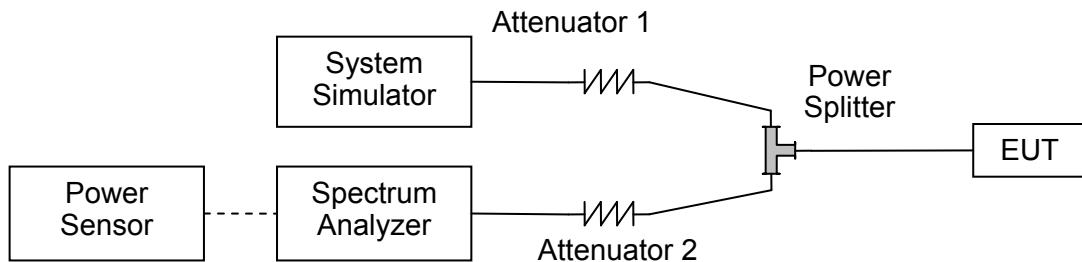
The EUT is coupled to the Spectrum Analyzer (SA) and the System Simulator (SS) with Attenuators through the Power Splitter; the RF load attached to the EUT antenna terminal is 50Ohm; the path loss as the factor is calibrated to correct the reading. The EUT is commanded by the SS to operate at the maximum output power. A call is established between the EUT and the SS.
