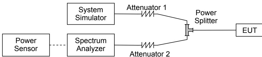
The EUT is coupled to the Spectrum Analyzer (SA) and the System Simulator (SS) with Attenuators through the Power Splitter; the RF load attached to the EUT antenna terminal is 50Ohm; the path loss as the factor is calibrated to correct the reading. The EUT is commanded by the SS to operate at the maximum output power. A call is established between the EUT and the SS.
