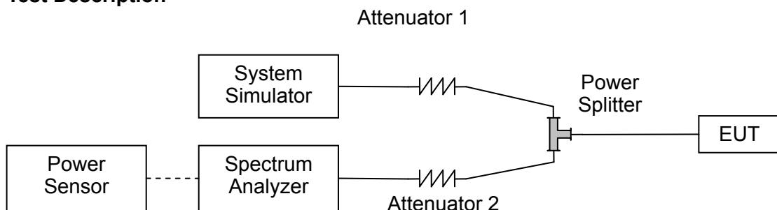
The EUT is coupled to the Spectrum Analyzer (SA) and the System Simulator (SS) with Attenuators through the Power Splitter; the RF load attached to the EUT antenna terminal is 50Ohm; the path loss as the factor is calibrated to correct the reading. The EUT is commanded by the SS to operate at the maximum output power. A call is established between the EUT and the SS.
