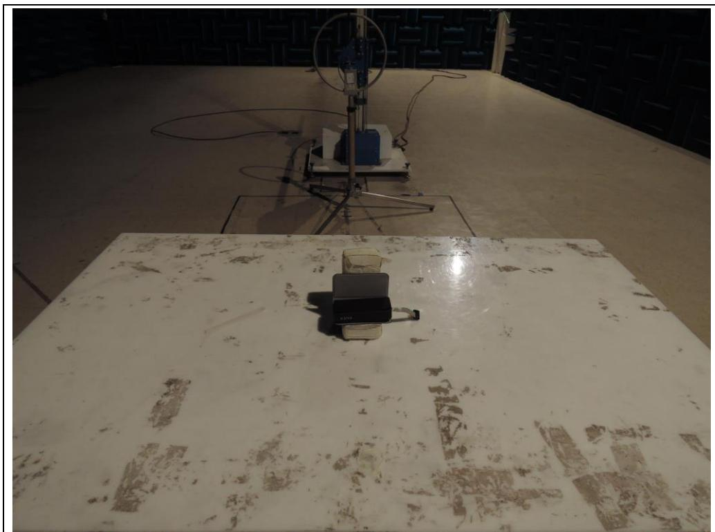
**Test Setup Photo of Radiated Measurement (below 1000MHz)**
