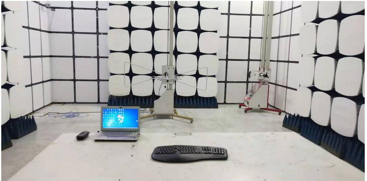
Test frequency from 1GHz-18GHz
