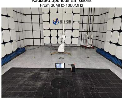
Radiated Spurious Emissions From 30MHz-1000MHz
