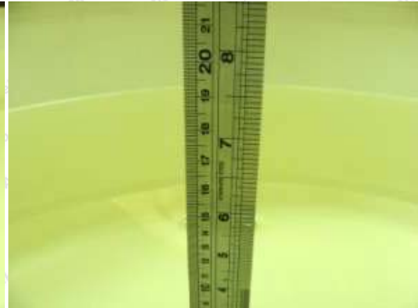
Photo of Liquid Height for Body SAR
