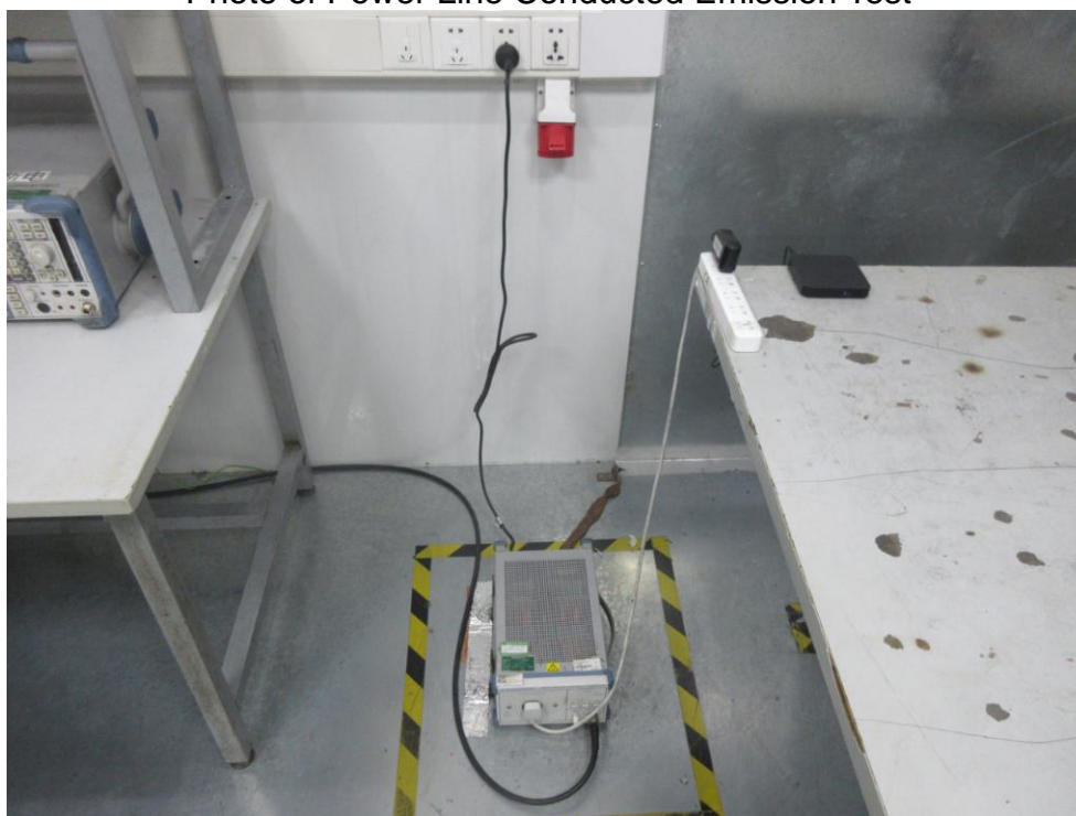
FCC ID: 2ACFBM6CX3-D4 Photo of Power Line Conducted Emission Test
