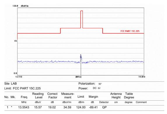
\*Note: Factor= Antenna Factor + Cable Loss
