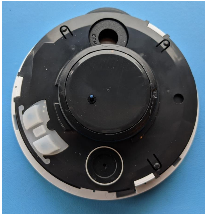
Internal cover installed over PCBAs on main enclosure soft plastic buttons and filter mesh
