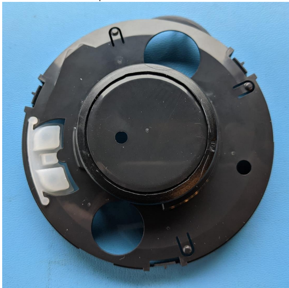
Internal plastic cover with soft plastic buttons and filter mesh
