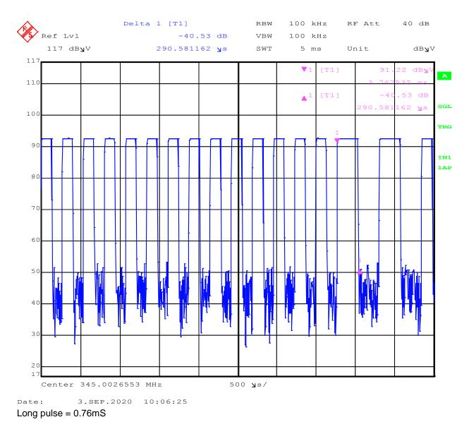
On Time = 0.27mS x 40 pulses + 0.76mS x 11 pulses On Time = 19.16mS Duty Cycle over 100mS = 19.16mS / 100mS = 0.1916
