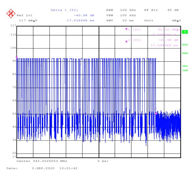
Number of short and long pulses in one pulse train 11 long pulses 40 short pulses
