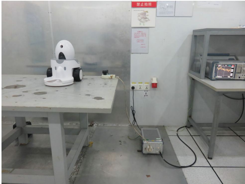
Photo of Conducted Emission Measurement
