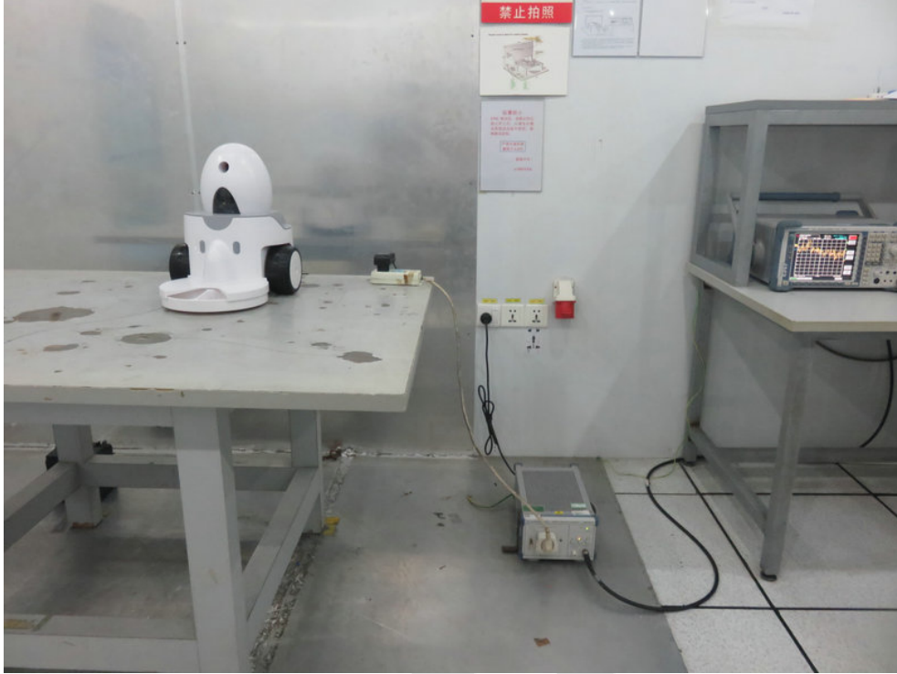
Photo of Conducted Emission Measurement
