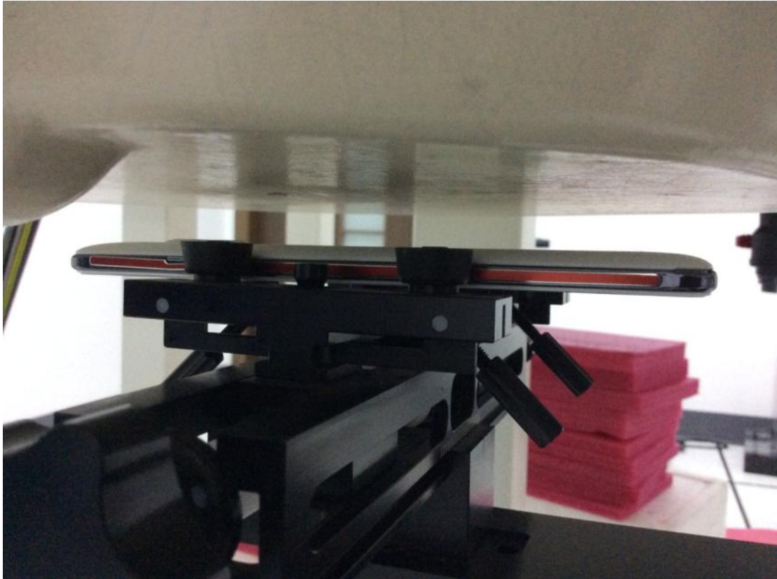
Test Setup Body Back with gap 10mm
