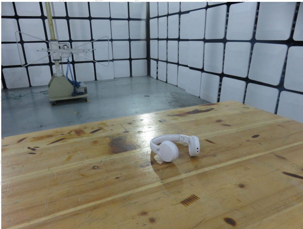
Photo of Radiation Emission Test
