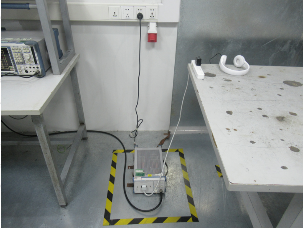
Photo of Conducted Emission Measurement
